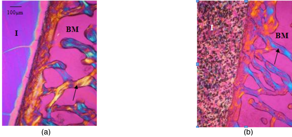
Figure 1. Polarized light micrographs after 24 weeks on (a) pure PLA and (b) GENESYS. I is implant, BM bone marrow, arrow the new-formed bone and bone trabeculae.
