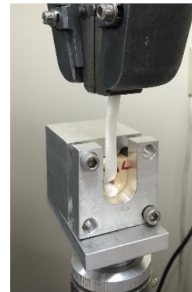
Figure 1: Tendon loaded at 90° on MTS machine.
